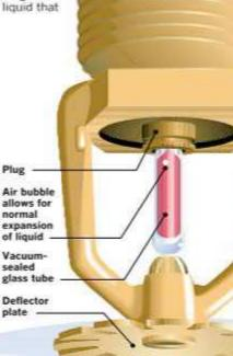
This liquid is designed to expand and break the tube at a certain temperature. The most common are designed to break at 155 degrees. In the average sized room, a 5mm diameter ampule will usually break in about one to one and a half minutes from contact with a heat source. Ampules as thin as 1mm are manufactured for a faster response time.
