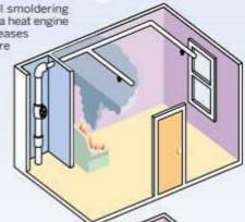
mechanism is heated to the required temperature, it trips and the water is released. The immediate cooling of the heat source usually prevents other sprinkler heads from activating. Often, one or two sprinkler heads are enough to control a fire.
